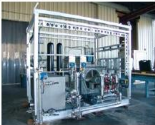
HPU/Lube Oil Skid
